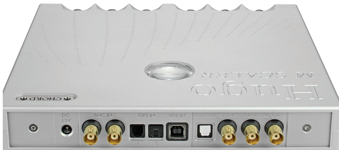
At left, two gold plated BNC digital inputs, two optical inputs and a USB for computer connection (centre). Then optical and BNC outputs, and right twin DBNC outputs for Chord Electronics products with matching DBNC inputs.
